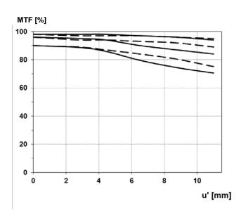
The Modulation Transfer (MTF) as a function of image height (u) and slit prientation (sagittal, tangential) has been measured with white light at spatial frequencies of R = 10, 20 and 40 cycles/mm.
